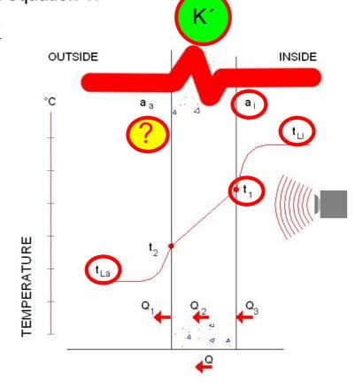
The outdoor surface conductivity a<sub>FAN</sub> is determined in equation 2:
