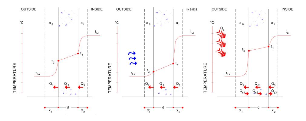
The variation of the surface temperatures in three cases: (a) theoretical, (b) in case of win (blue arrows) and (c) in case of solar radiation (red arrows)
