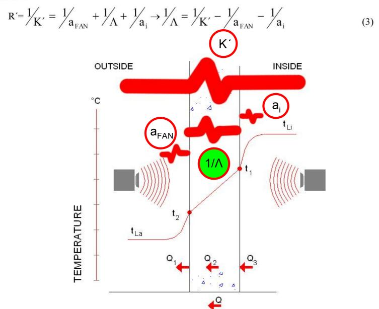
The thermal resistance of a building's envelope according to the Greek Standards for the thermal insulation of buildings is given in equation 4:
