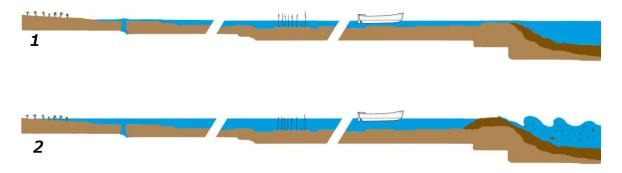
**Figure 3**: Schematic longitudinal section showing the open flow to the sea (1) and the potential blockage of the river's mouth by debris (2)
