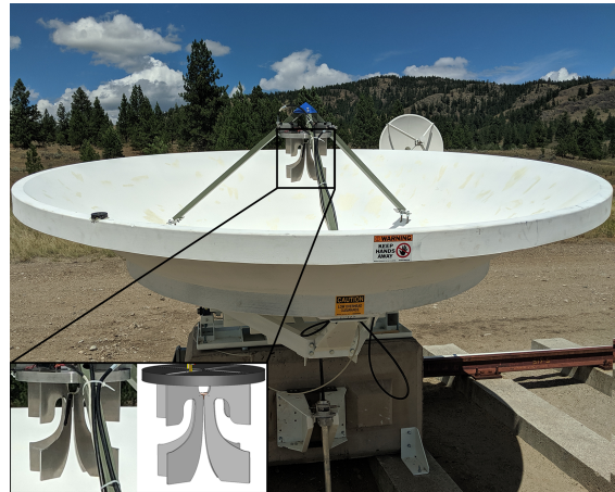
Figure 5: Prototype composite dish, deployed at Canada’s Dominion Radio Astrophysical Observatory (DRAO). A UWB feed is mounted at the focus, with detail shown inset at lower left, alongside CAD model.
