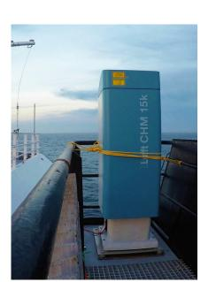
Lufft CHM 15k is a near-infrared (1064 nm) ceilometer with a range of 15 km.
