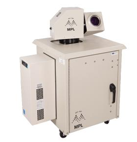
MiniMPL is a visible spectrum (532 nm) dual-polarisation lidar with a range of 30 km.
