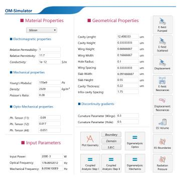
Fig. 2: Snapshot of the graphic user interface of the developed application. Four sections can be easily distinguished: The *Material Properties* section, in which it is possible to specify the physical characteristics of the sample taken into examination, the *Geometrical Properties* section, the *Input Parameters* section, in which frequencies (both optic and mechanical) and the laser input power are defined and the *Evaluation & Results* section.
