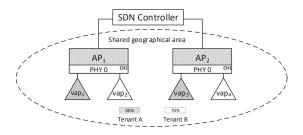
Fig. 2: Two APs sharing the wireless medium due to close vicinity. The APs provide *vaps* for two tenants (A, B) that have been assigned shares of 30% and 70%, respectively.
