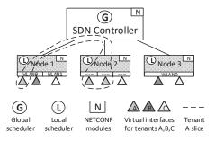
Fig. 1: Our network architecture is composed of APs with physical interfaces, on top of which virtual interfaces (*vifs*) are instantiated for different tenants. The SDN controller manages the *vifs* and configures the APs to apply the Wi-Fi slicing.
