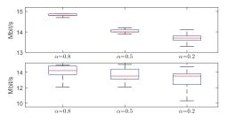
Fig. 3: Box plots showing the throughput, with the median, 1st and 3rd quartiles (lower/upper box limits), and min. and max. values (lower/upper whiskers) for the continuous case (top) and with interference (bottom).
