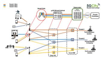
Fig. 3. 5GCity Neutral Host model for network slicing
