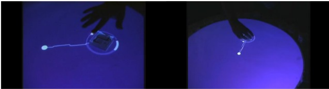
Figure 4.2: Controlling a reactable object by touching with a finger (left) and by rotating (right)
