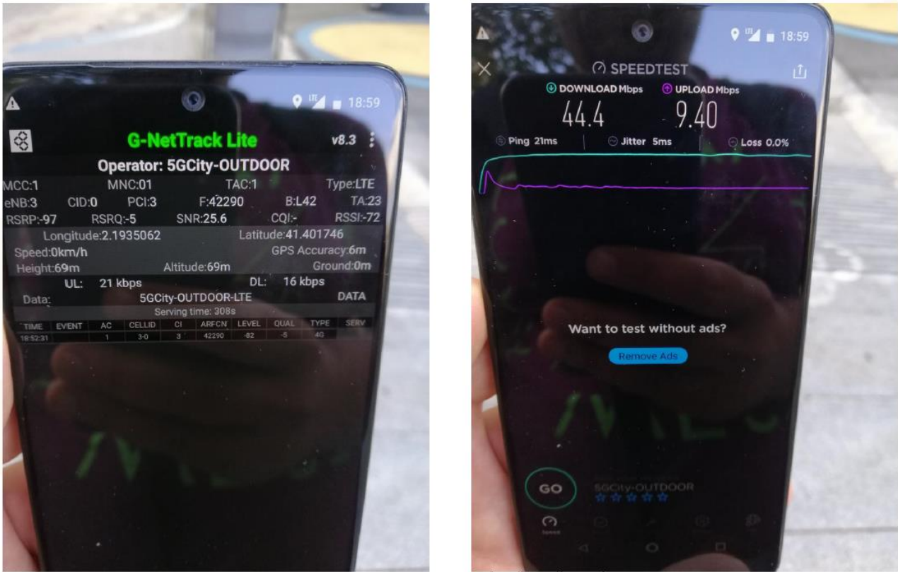
Figure 28: RAN SNR and SpeedTest in Barcelona @22 district (measurement point 2).
