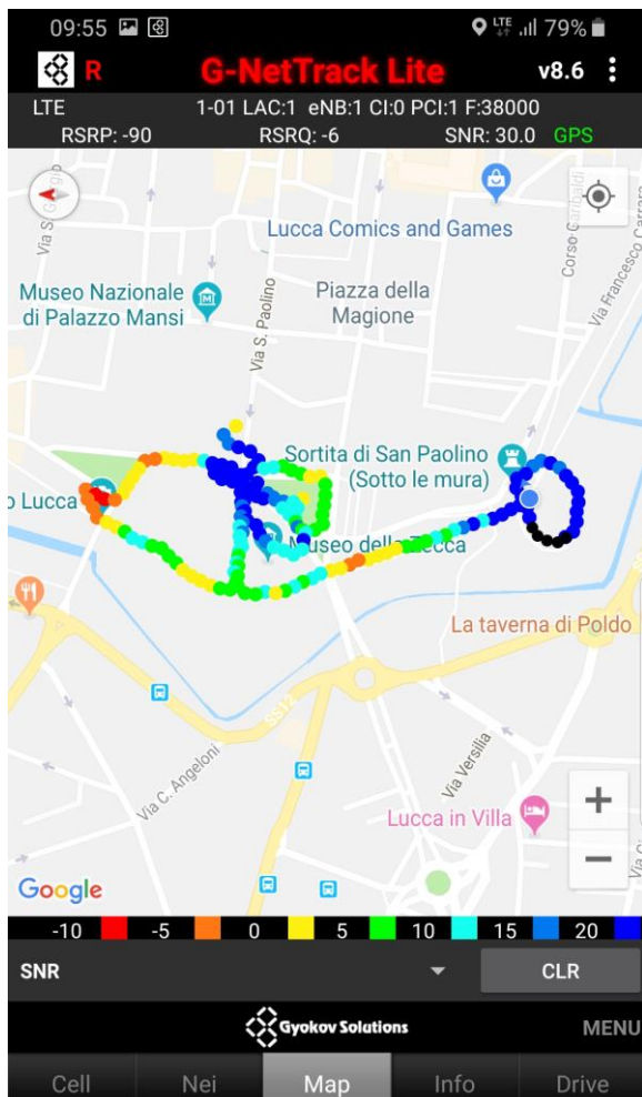
Figure 34: 5GCity LTE coverage in Lucca (High SNR values in blue dots, closer to 5GCity SCs).
