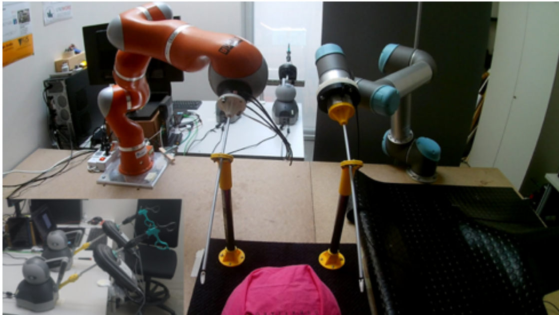
Figure 3: Setup for the preliminary validation of the bilateral teleoperation architecture for the assistant surgeon.
