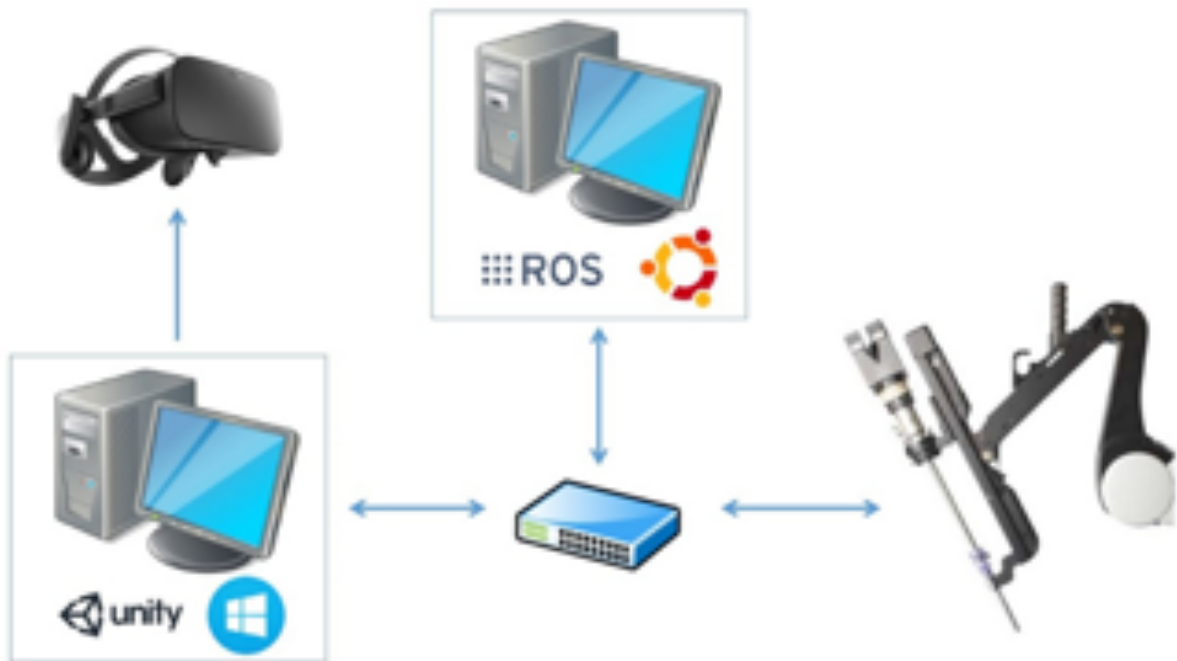
Figure 11: Schematic overview of the setup for augmented reality.
