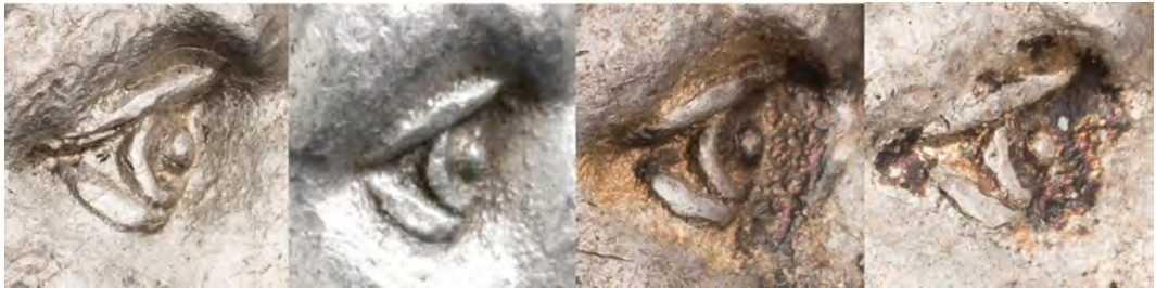
Figure 3. Development of die rust on A5 (Cat. Nos. 15, 18, 19 and 20).
