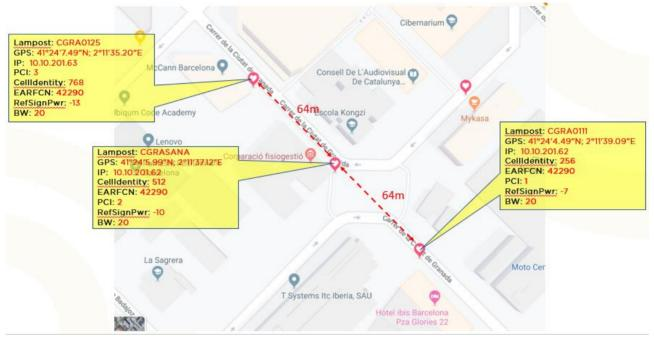
Figure 9: 5GCity Small Cells deployment in Barcelona
