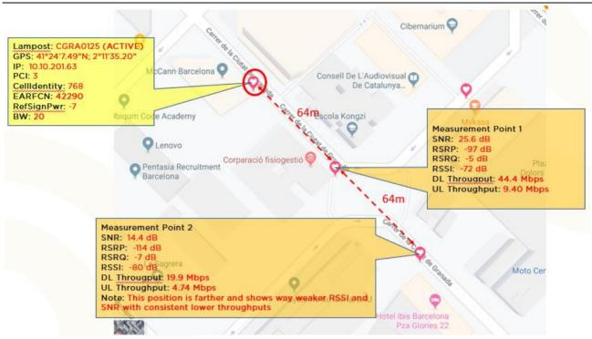
Figure 10: 5GCity Small Cell CGRA0125 initial throughput at range validation
