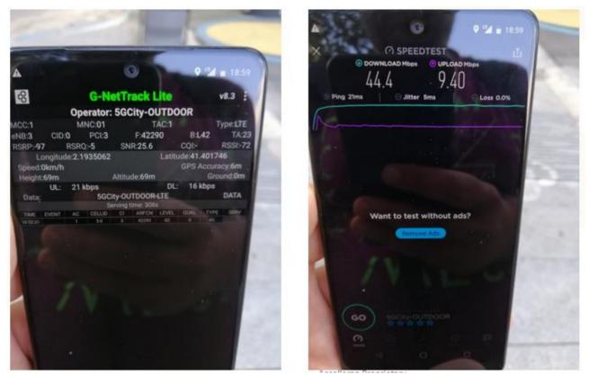
Figure 11: 5GCity GNetTracker and SpeedTest data for CGRA0125 lamppost with UE in Position 1
