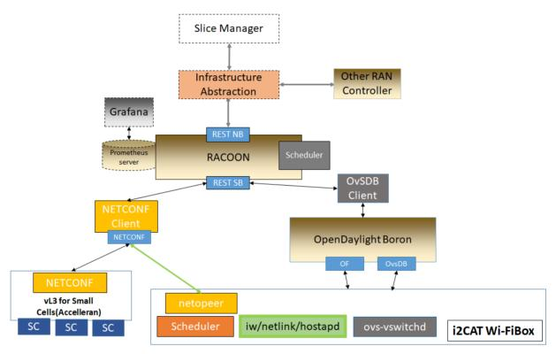
Figure 4: Overview of the software components forming the RAN virtualization framework.
