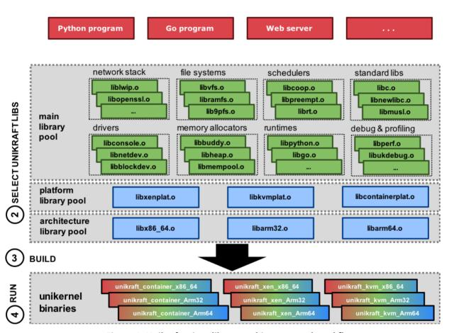
Figure 1. Unikraft micro-library architecture and workflow.
