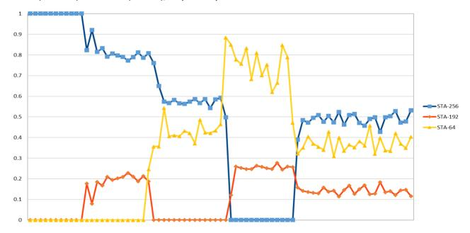
Figure 8: Results showing the airtime consumed by each UE when applying the Wi-Fi scheduler with a setting of 50% (STA-256), 12.5% (STA-192) and 37.5% (STA-64)
