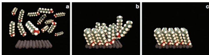
FIGURE 3. Schematic Depiction of SAM Formation of a Monolayer-thick Film.
