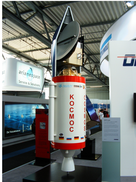
Figure 3: Mockup of a Kosmos 3M second stage with a model of a German SAR-Lupe reconnaissance satellite mounted on top of it (source: Wikimedia )
