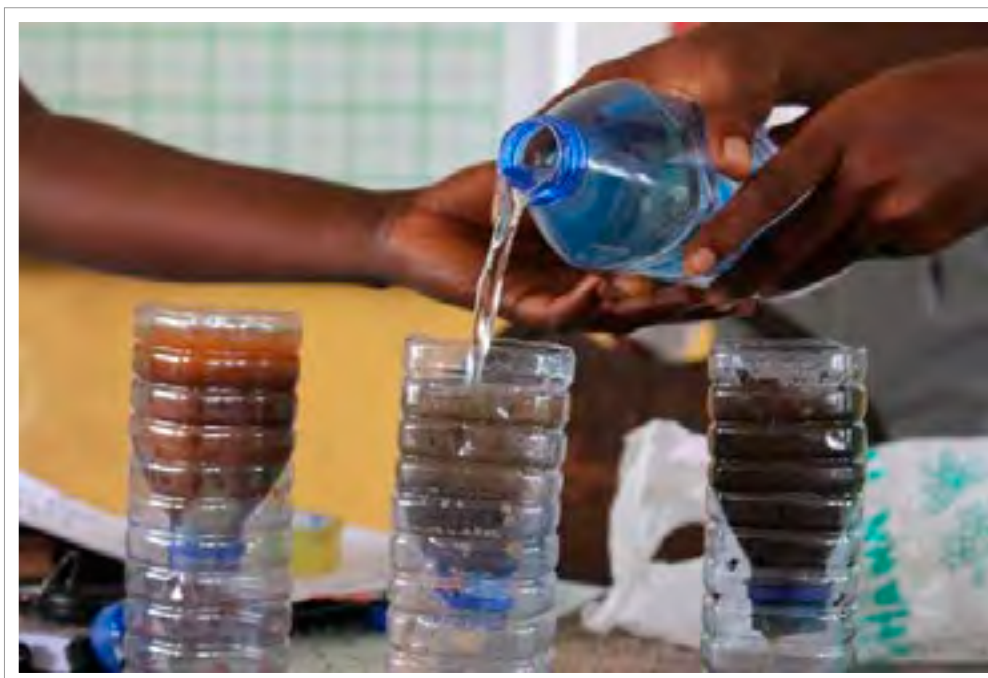
Figure 106. Testing water retention
