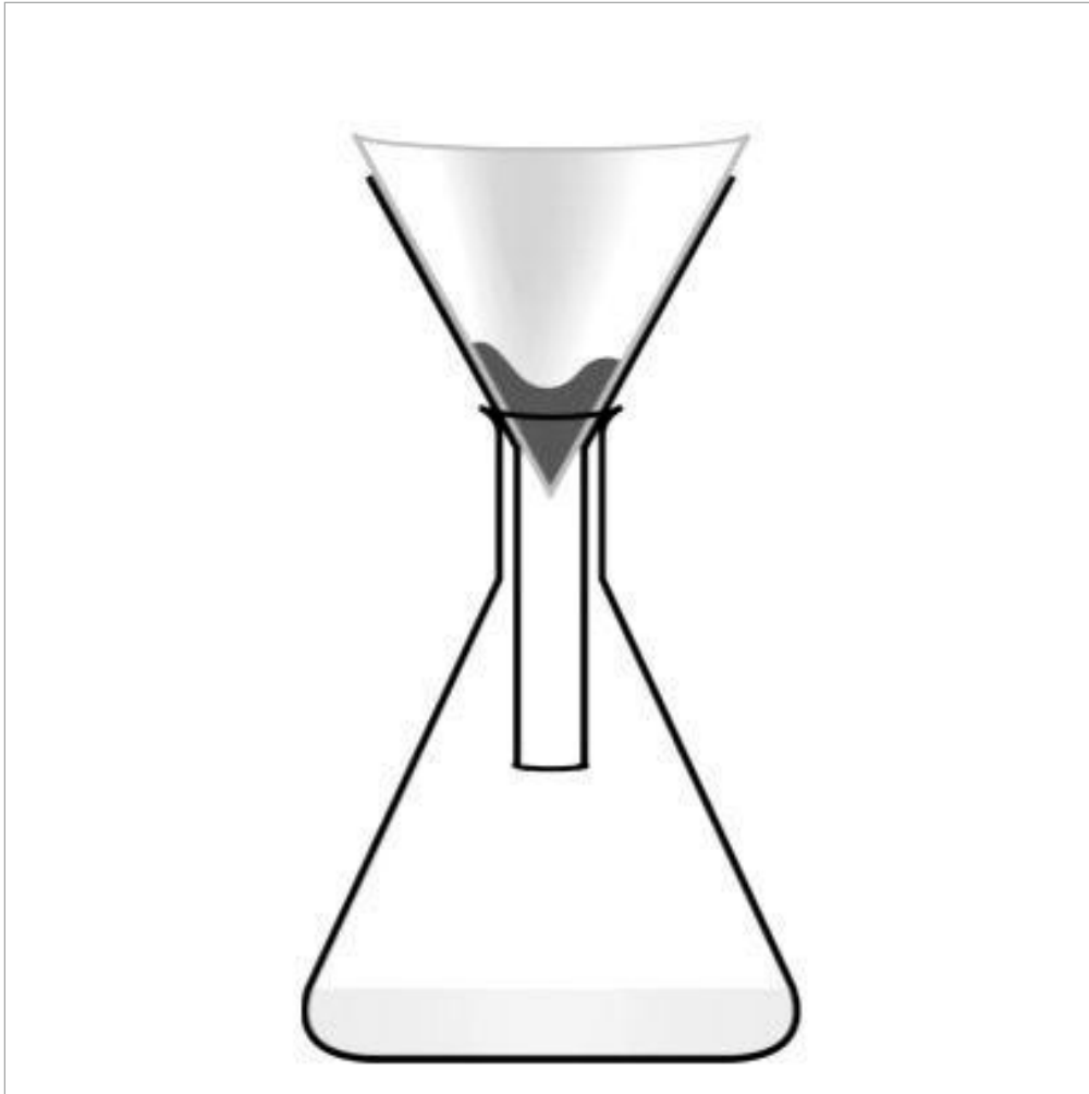
Figure 39. Filtering a mixture of salty water and sand
