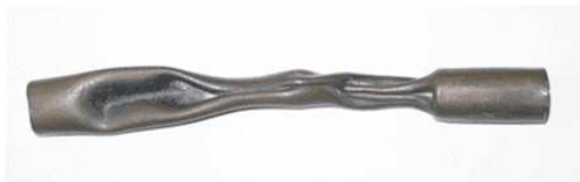
FIGURE 1. Copper Pipe Crushed by the Z-Pinch from a Lightning Strike (Image credit: Univ. of Sydney)
