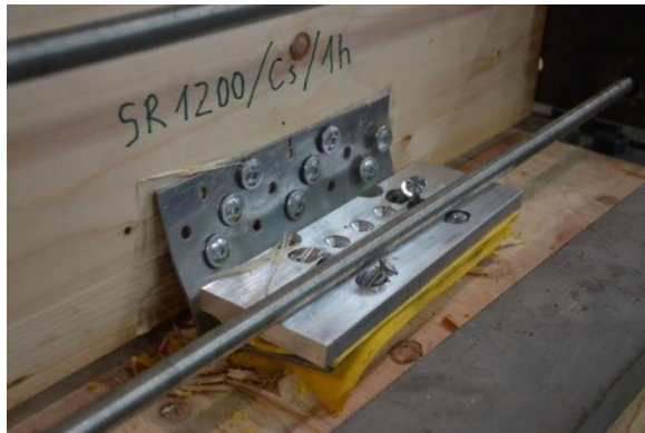
c. Embedding and withdrawal of screws from the floor and wall panel (insulated specimen)
