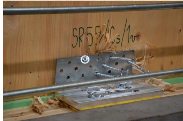
b. Embedding and withdrawal of screws from the wall panel (insulated specimen)
