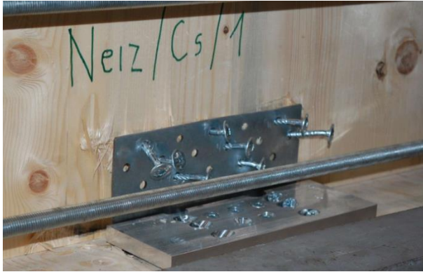
a. Embedding and withdrawal of screws from the wall panel (uninsulated specimen)
