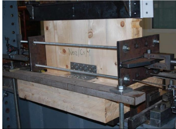
Figure 2. Test specimen - CLT wall and floor panel connected with angle bracket without insulation bedding
