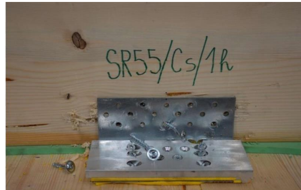
d. Embedding, withdrawal and shear failure of screws in the wall panel (insulated specimen)
