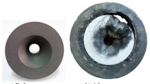
a) Before test b) After test Fig. 16. Pictures of the CN-SF-1 nozzle.
