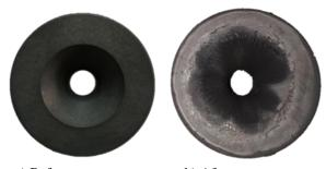
a) Before test b) After test Fig. 17. Pictures of the CN-SF-2 nozzle.
