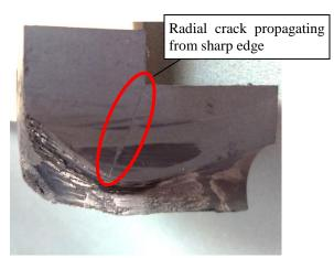
Fig. 19. Picture of the cut section of CN-SF-1 nozzle correspondingly to the radial crack.
