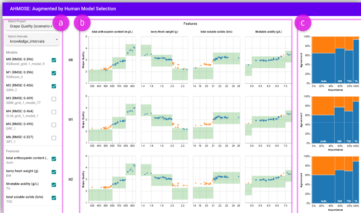
Figure 7: The AHMoSe interface: a) the sidebar controls to select the use case, intervals, models and features to be visualized, b) the scatter plots highlight the comparisons between models' predictions (orange and blue dots) and domain expert knowledge (green rectangles), c) the Marimekko charts indicate the importance of each feature according to the given model, and the agreement between the model and domain expert knowledge.
