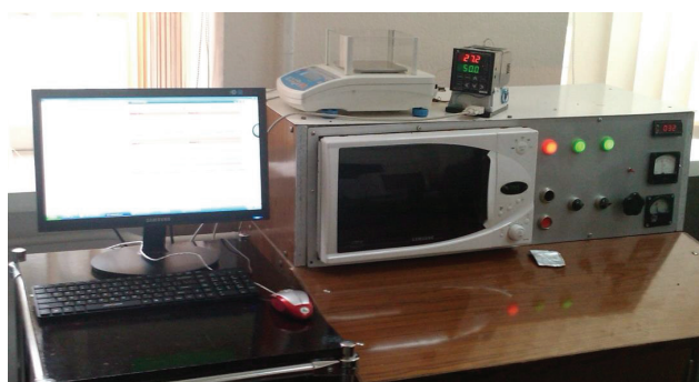
Fig. 2. A computerized stand for the study of the dehydration kinetics in an electromagnetic infrared field
