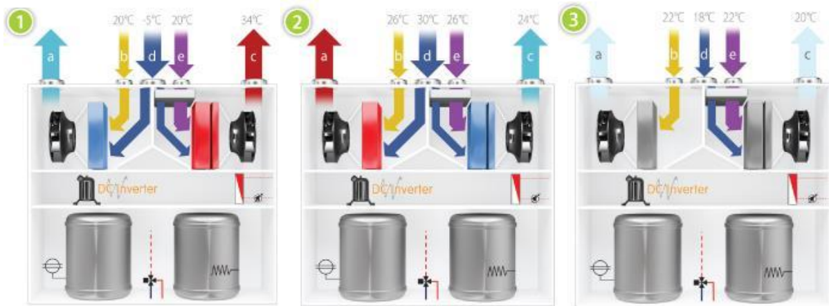
Figure 14 – Working modes of the Elfopack in 1) heating, 2) cooling and 3) free cooling mode http://www.clivetlive.com/en/web/quest/elfopack1
