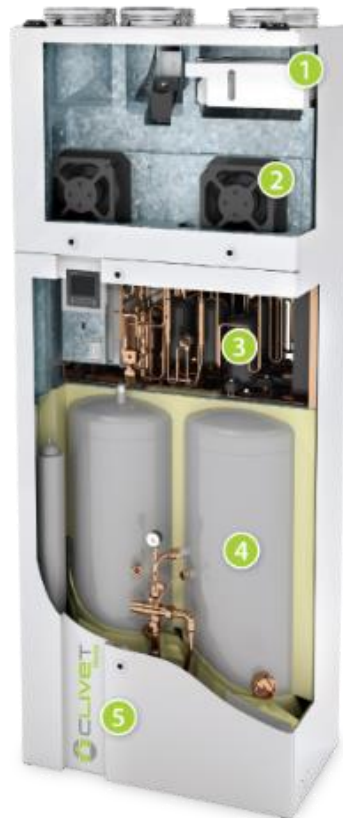
Figure 15 – 3D view and section of the Elfopack ( http://www.clivetlive.com/en/web/quest/elfopack1 )
