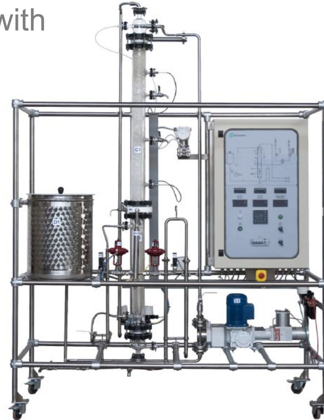
1m (80mm ID) packed column (Raschig rings)
