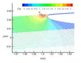
Fig. 15. Pressure coefficient field of the single-phase APR simulation involving 8 refinement levels at time t = 0.02 s. The size of the pressure gauge  $P_{18}$  is depicted.
