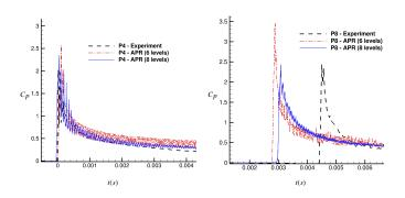
Fig. 16. Comparison between experimental data and SPH APR simulations (single-phase model): pressure time histories for probes P4 and P8.
