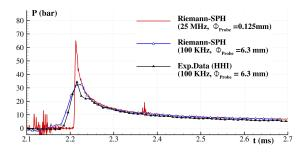
Fig. 6. Vertical impact of a flat panel: SPH pressure time histories versus experimental data. The SPH signal recorded using the size of the experimental pressure gauges and filtered at 100 kHz is also shown.
