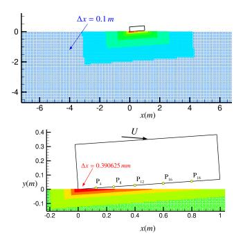
Fig. 14. Sketch of the single-phase simulation involving 8 refinement levels (top: global view, bottom: zoomed view). Colors refer to refinement depth.
