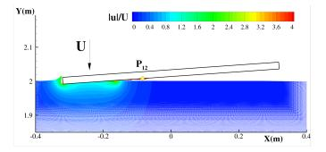
Fig. 1. Vertical impact of a flat panel. Colors are representative of the SPH velocity intensity. Pressure probe number 12, which is the gauge used for the comparison with the experimental data, is also depicted.
