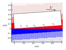
Fig. 17. Sketch of the two-phases simulation involving 8 refinement levels (top: refinement levels, bottom: phase configuration)
