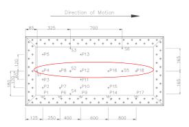
Fig. 13. Top view of the plate. Red ellipse shows pressure probes considered for 2D SPH simulations (measures are in mm).
