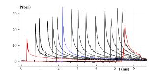
Fig. 7. Vertical impact of a flat panel: experimental data for the pressure time histories on a row of probes (not equispaced). The time history from the first and last probes on the panel impacting the water are colored in red. The time history in blue is from probe  $P_{12}$ , used in the previous figures for comparison with the SPH solution.
