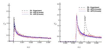
Fig. 19. Comparison between experimental data and SPH APR simulations (two-phases model): pressure time histories for 4 different probes
