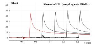
Fig. 8. Vertical impact of a flat panel: SPH pressure time histories on a row of probes. The original SPH signals have been filtered with a MAF at 100 kHz as in the experimental signals. The time history from the first probe on the panel impacting the water is colored in red.
