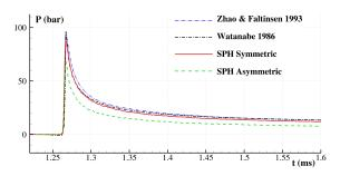
Fig. 12. Vertical impact of a flat panel: pressure time histories of symmetric (solid line) and asymmetric (dashed) solutions measured at 0.16 m from the left-hand edge of the panel. Analytical solutions by [21] (dash-dot line) and by [10] (dash dot-dot line) are also reported.
