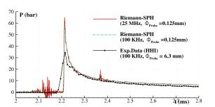
Fig. 5. Vertical impact of a flat panel: SPH pressure time histories versus experimental data. The SPH signal is filtered with a running average filters (MAF) at 100 kHz (dashed-dotted line).
