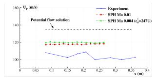
Fig. 9. Vertical impact of a flat panel: Peak propagation velocity  $U_P$  calculated on several positions along the panel for the experiment (triangles), SPH simulation at Ma=0.01 (circles) and Ma=0.004 (squares), and analytical value from potential flow theory (dashed line). The origin of the x-axis is set at the left-hand edge of the panel.
