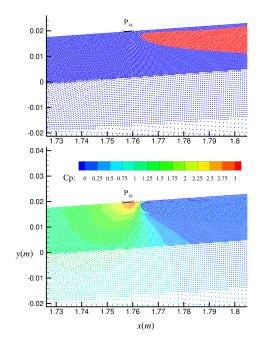
Fig. 18. Phase configuration (top) and pressure coefficient field (bottom) of the two-phases APR simulation involving 8 refinement levels at time  $t = 0.024 \ s$ . The size of the pressure gauge  $P_{18}$  is depicted.
