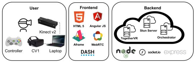
Figure 1 – Overview of the TogetherVR application framework.
