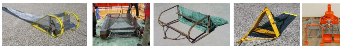
Figure 1. Sampling devices A-D routinely used for zoological sampling. A) RP-sledge, B) Detritus sledge, C) Agassiz trawl, D) Triangular dredge. E) Shipek grab, samples taken for sediment analysis only.
