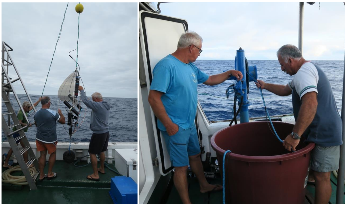
Fig. 1. Image of the drift-cam system being deployed from the side of the vessel and the crew of N/I Arquipélago maneuvering the hydraulic winch to correctly position the system with respect of the seabed.
