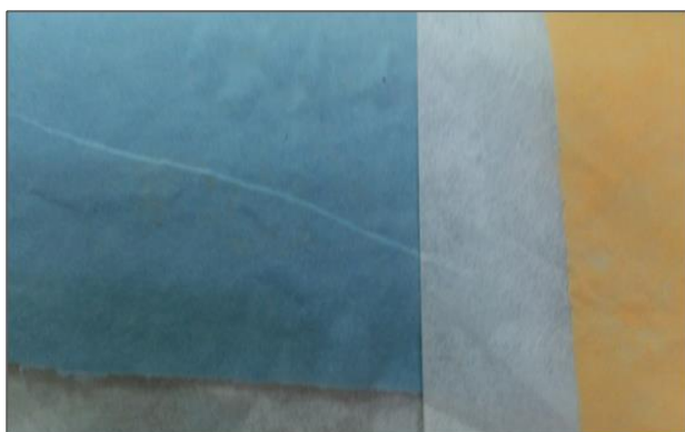
Figure 9. Paper sheets prepared on leaf-casting machine.
