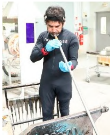
(c) Blowing: The technique of forming an object by inflating a gather or gob of molten glass on the end of a blowpipe.
