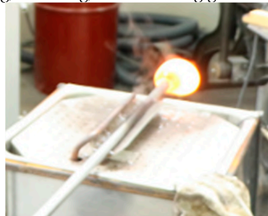
(b) Gather, or gob: A mass of molten glass collected at the end of a blowpipe, pontil, or gathering iron.
