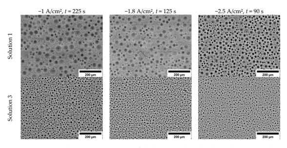
**Figure 2.** Scanning Electron Microscopy images of cobalt coatings obtained under a galvanostatic mode at various deposition conditions, but the same value of charge passed (q = 180 C).
