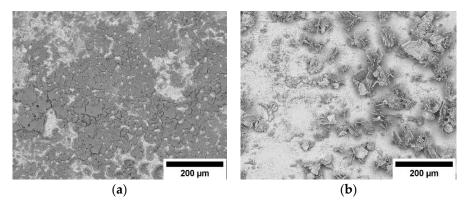
**Figure 1.** SEM images of Co coatings deposited under galvanostatic conditions, at cathodic current density j = 2.5 A/cm<sup>2</sup>, deposition time t = 60 s. The composition of solutions: (**a**) 0.2 M CoCl<sub>2</sub>; (**b**) 0.2 M CoSO<sub>4</sub>.
