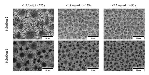
**Figure 3.** Scanning Electron Microscopy images of cobalt coatings obtained under a galvanostatic mode at various deposition conditions, but the same value of charge passed (q = 180 C), from solutions containing isopropyl alcohol.
