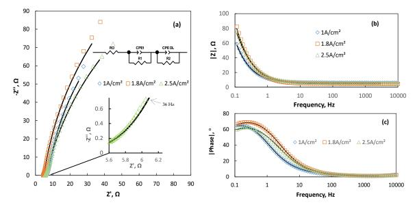
**Figure 7.** EIS data of cobalt foams measured in 0.1 M Na<sub>2</sub>SO<sub>4</sub> at -1.0 V vs Ag/AgCl, foams deposited from solution 4, q = 180 C, EIS data represented in: (a) Nyquist's coordinates, (b) Bode modulus, and (c) Bode phase modulus coordinates. The equivalent electric circuit used for fitting is presented in the insert; points–experimental data, solid lines–results of fitting to the shown equivalent electric circuit.
