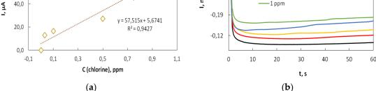
**Figure 10.** Calibration curve for sensors (**a**) and typical chronoamperometric curves for free chlorine detection in acetic acid buffer (**b**).
