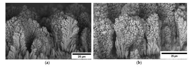
**Figure 6.** SEM images of cobalt foams cross-sections deposited under galvanostatic mode, from solution 4: (a) j = 1 A/cm<sup>2</sup>, t = 225 s; (b) j = 2.5 A/cm<sup>2</sup>, t = 90 s.
