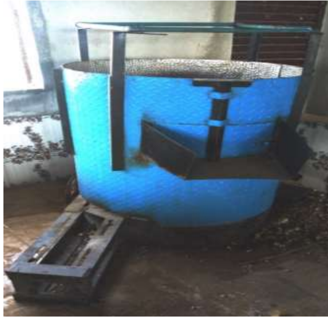
Plate 1. Pictorial View of the Rotary Cassava Peeling Machine.
