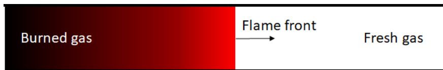
Figure 8: Schematic representation of flame propagating in a tube
