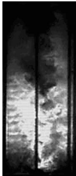
Figure 14: MIE scattering of the suspension at 40,9 ms from the beginning of the dispersion (Bozier 2004)
