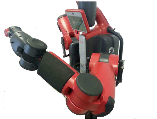
(b) Sensorized link mounted on the real robot and covered with a conductive ground plane.
