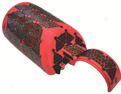
(a) Real robot link covered with robot skin.
