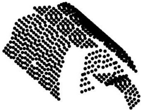
(b) Placement of the taxels obtained from the spatial calibration of the skin.
