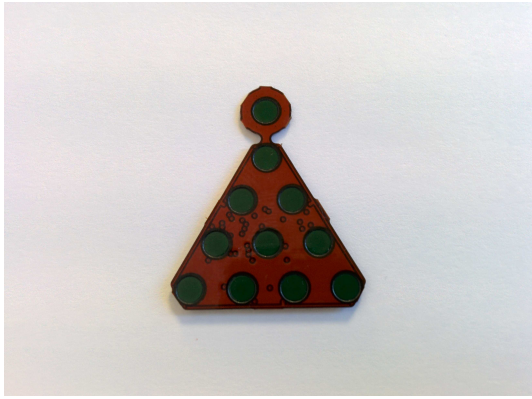
(a) Triangular module of the robot skin. The diameter of each taxel is 3.5\text{ mm} , with a pitch of 8\text{ mm} among nearby taxels.
