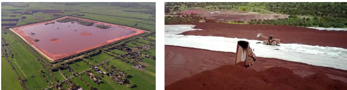
Figure 27 Typical Bauxite residue slurry storage (left) and filtercake storage at Mytilineos (right)
