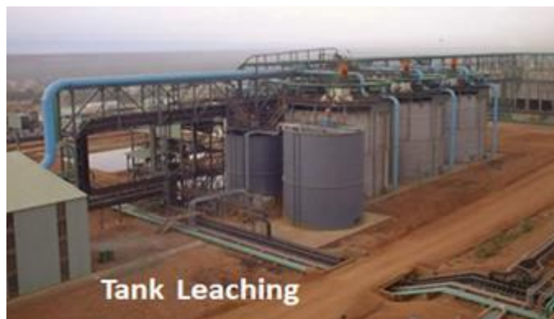
Figure 24 Picture of the tank leaching processes implemented at the Kasese Cobalt Company site in Uganda.
