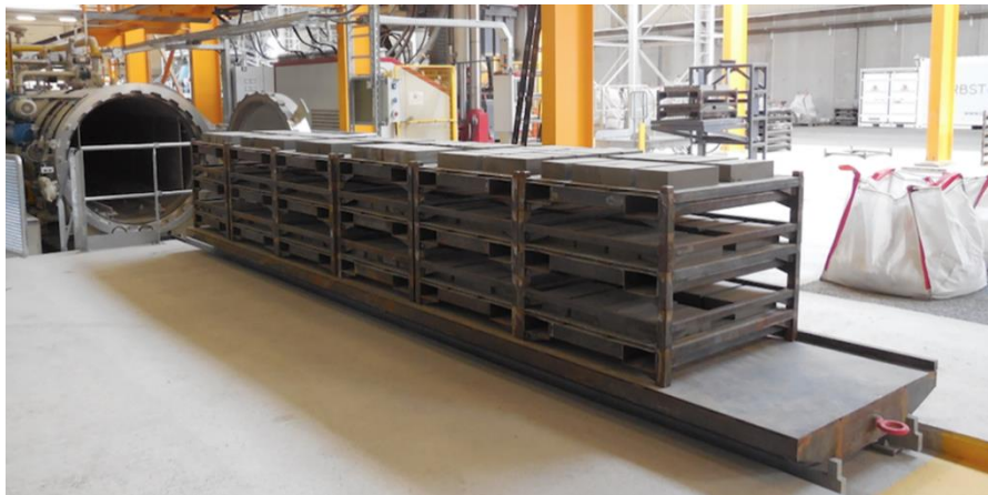
Figure 23: Production of carbstone bricks in the Orbix pilot facility in Belgium
