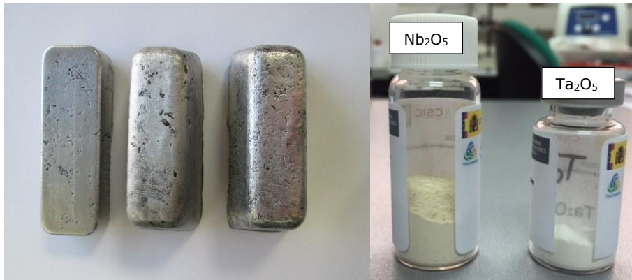
Figure 19 Products resulting from the R&D projects: tin ingots (left) and Nb and Ta oxides (right)
