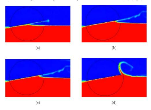
Figure 13 Evolution of fluid free surface during the plate impact
