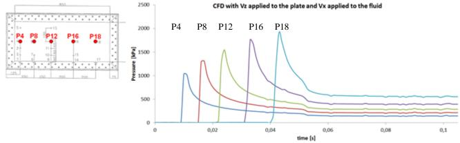
Figure 14 CFD results (filtered) for Vz=1.5 m/s, Vx= 40 m/s & Pitch angle = 10 deg.
