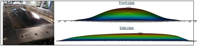
Figure 20. (Left): extremely flexible aluminum plate (t=0.4 mm) tested in SARAH project (Right). Test vs simulation comparison of the permanent deformation on a 0.4 mm aluminum panel result of ditching loads.
