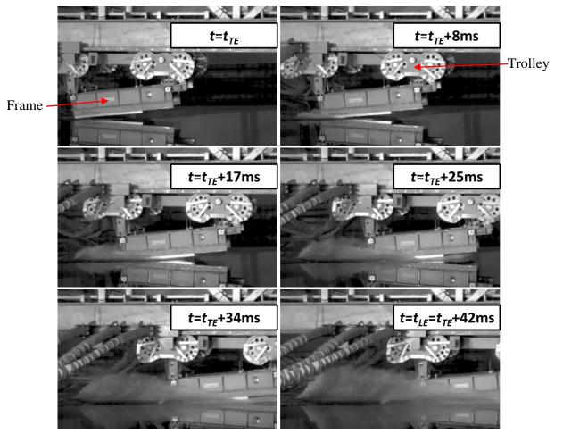
Figure 4: Pictures illustrating the guiding structure, the trolley and the specimen at impact phase
