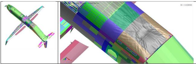
Figure 22. Left: aircraft structural deformation due to ditching pressures.. Right: local detail zoom.
