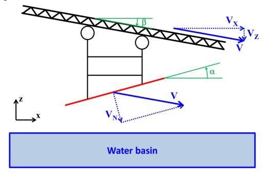
Figure 6: Initial ditching conditions sketch
