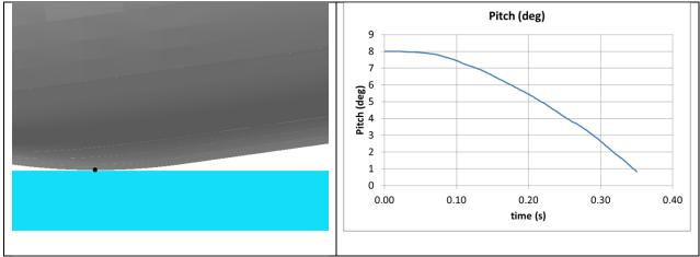
Figure 21. Left: aircraft geometry at first impact point. Right: aircraft pitch time history evolution in ditching.
