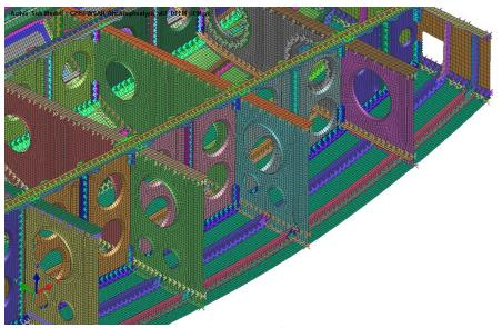
Figure 19. Zoom of the detailed bottom fuselage model to illustrate mesh size.
