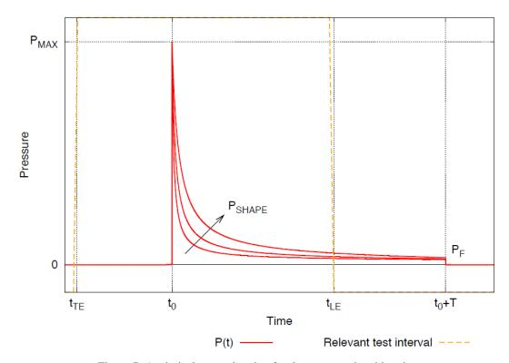
Figure 7: Analytical approximation for the pressure time histories
