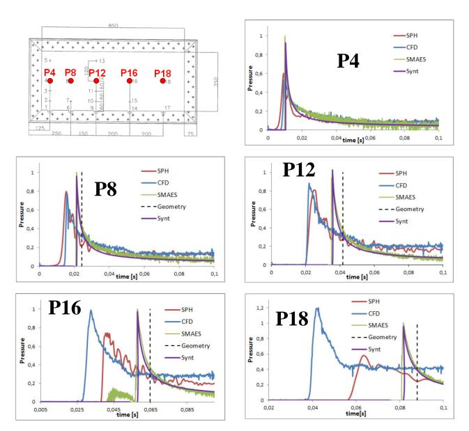
Figure 17 Comparison of different normalized ditching pressures numerical simulation methodologies with test results (Vx=40 m/s, pitch 10 degrees)
