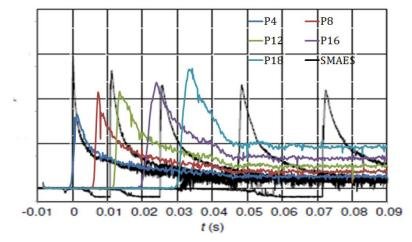
Figure 15 Comparison of CFD results (unfiltered) Vs. SMAES test (Vz=1.5 m/s, Vx=40 m/s, Pitch =10 deg.)
