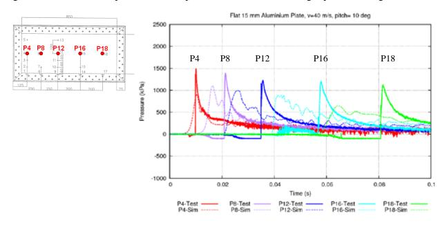
Figure 11: Comparison of SPH pressures versus SMAES rigid plate ditching test
