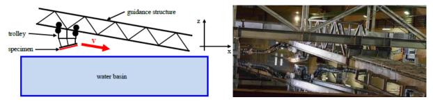
Figure 2: Schematic sketch of the guided ditching test setup
