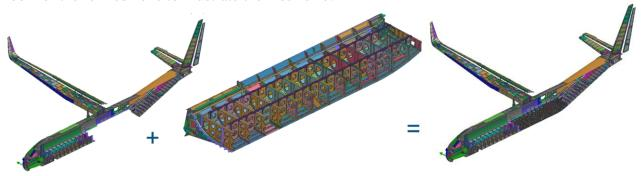
Figure 18. Global FEM model. Detailed bottom fuselage model. Integrated model for ditching calculations.
