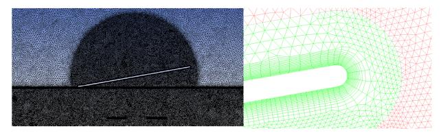
Figure 12 (Left) SMAES guided ditching test model implemented in ANSYS Fluent (2D). (Right) CFD Mesh
