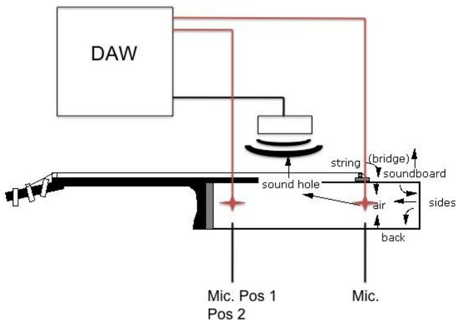
Figure 3.3 : Signal chain and microphone/loudspeaker positioning.
