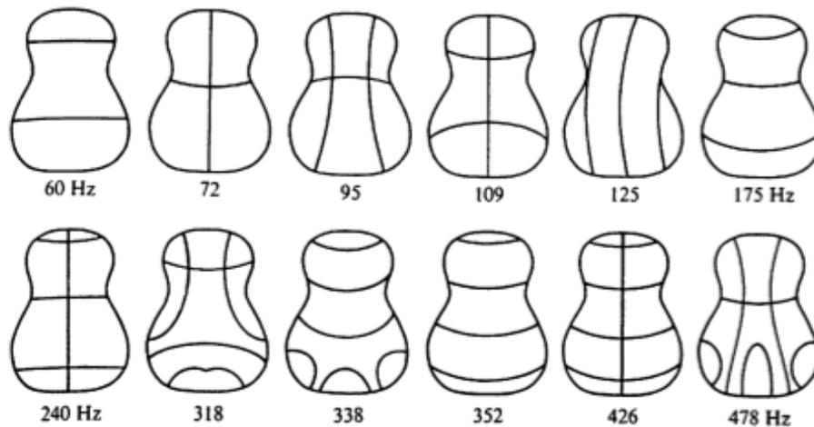
Figure 2.6 : Vibration modes of guitar without bracings.
