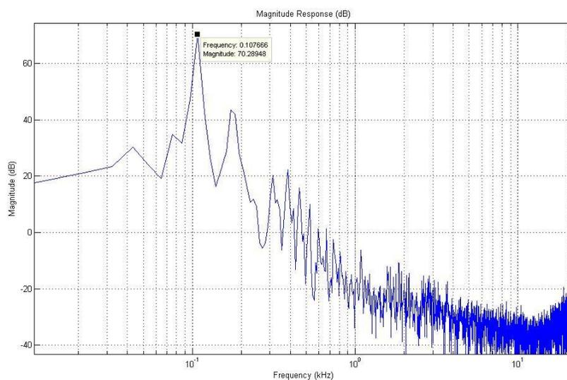
Figure 3.2 : Impulse response of Experimental Modal Analysis of point 14, Torres 625
