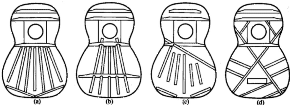
Figure 2.10 : Bracing designs
