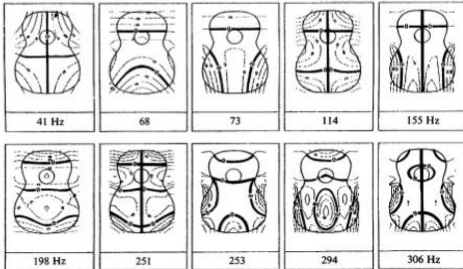
Figure 2.7 : Vibration modes of plates with bracings
