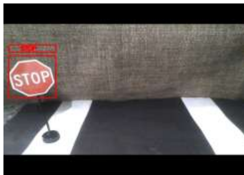
Fig.23: Stop sign detected using HaarCascade
