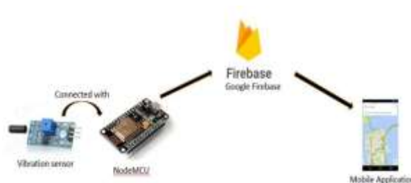
Fig.20: Working of RADS system
