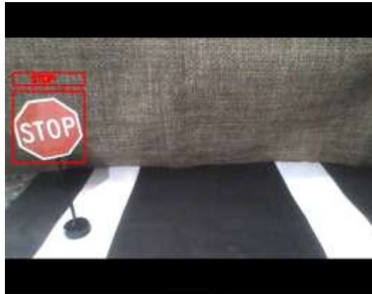
Fig.19: Sign Board detected with Harcascade
