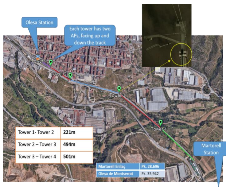
Figure 4.6: Demonstration configuration for railway services
