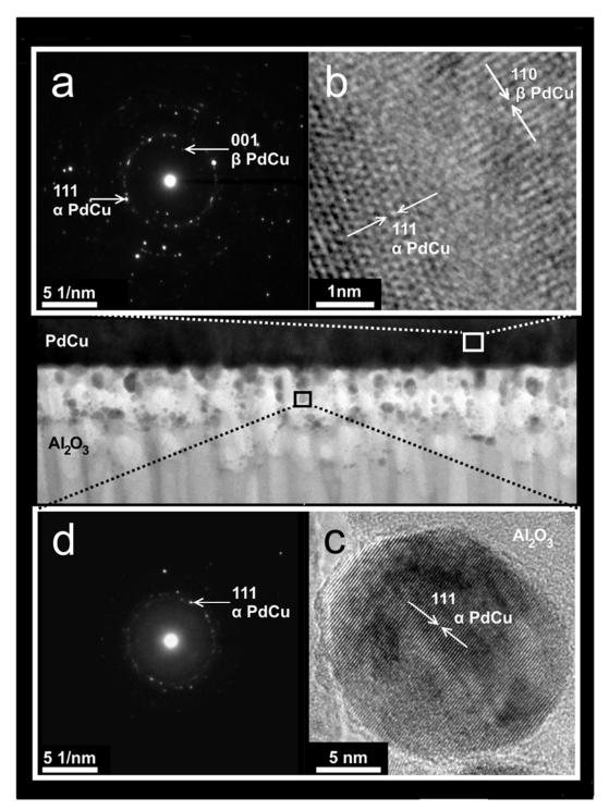
Fig. 5 Fragments of the SAED (a, d) and TEM image (phase contrast) cross FIB section of  $Al_2O_3/PdCu$  from the region of the PdCu film remote from the interphase boundary with the substrate (b) and inside the pore (c).
