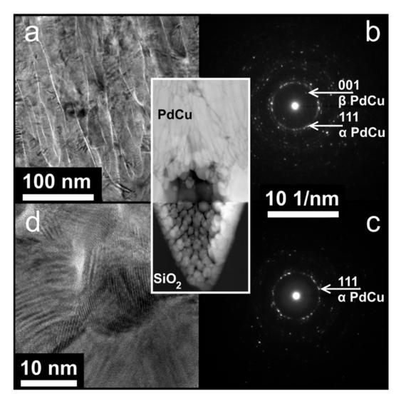
Fig. 3 Fragments of the SAED (b, c) and TEM image of the structure (a, d) cross FIB section of PdCu crystallites in the region remote from the interphase boundary with SiO<sub>2</sub> (c, d) and inside the pore (a, b). Sample type **II**.
