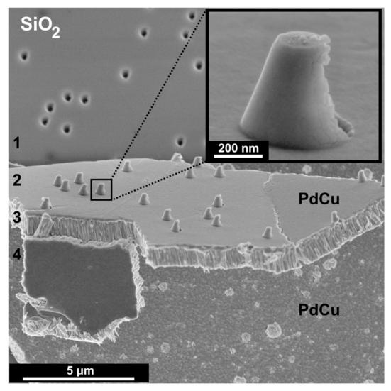
*Fig. 1 SEM image of the sample type I*: *porous surface of SiO*<sup>2</sup> *after peeling of the PdCu film (1), the surface of the PdCu film on the substrate side (2), its fracture (3) and growth front (4).*
