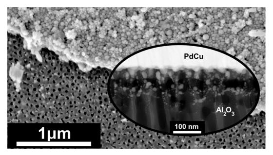
Fig. 4 SEM image of the fracture of the PdCu film on the surface of porous alumina (a) and the TEM image (in the Z-contrast recording mode) of the cross FIB section of the Al<sub>2</sub>O<sub>3</sub>/PdCu (b).
