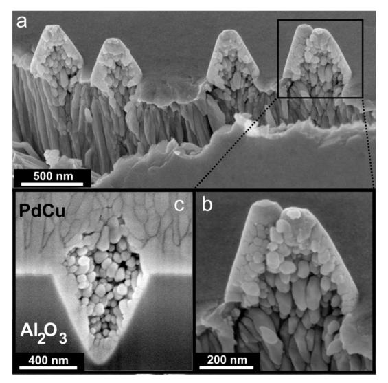
Fig. 2 SEM images of the sample type **II**: the interphase surface of PdCu from the SiO<sub>2</sub> side (a); extracted "imprint" of pores (b); cross section of FIB heterostructure Si/SiO<sub>2</sub>/PdCu (c).
