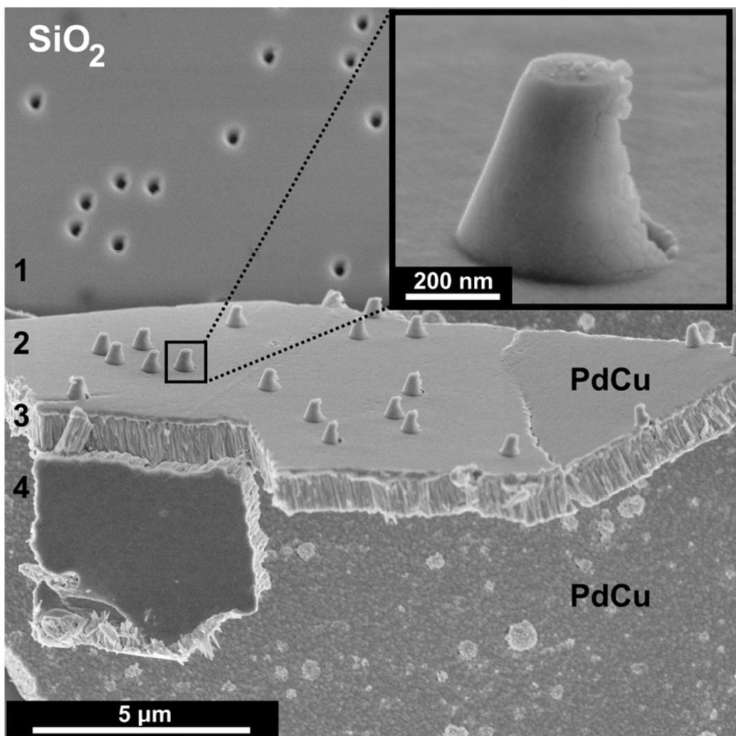
Fig. 1 SEM image of the sample type I: porous surface of  $\text{SiO}_2$  after peeling of the PdCu film (1), the surface of the PdCu film on the substrate side (2), its fracture (3) and growth front (4).
