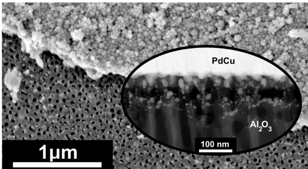
Fig. 4 SEM image of the fracture of the PdCu film on the surface of porous alumina (a) and the TEM image (in the Z-contrast recording mode) of the cross FIB section of the Al<sub>2</sub>O<sub>3</sub>/PdCu (b).
