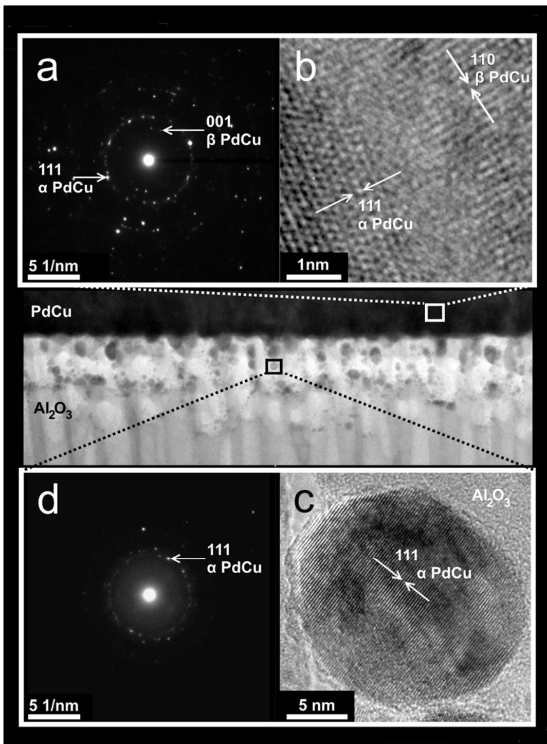
Fig. 5 Fragments of the SAED (a, d) and TEM image (phase contrast) cross FIB section of  $\text{Al}_2\text{O}_3/\text{PdCu}$  from the region of the PdCu film remote from the interphase boundary with the substrate (b) and inside the pore (c).
