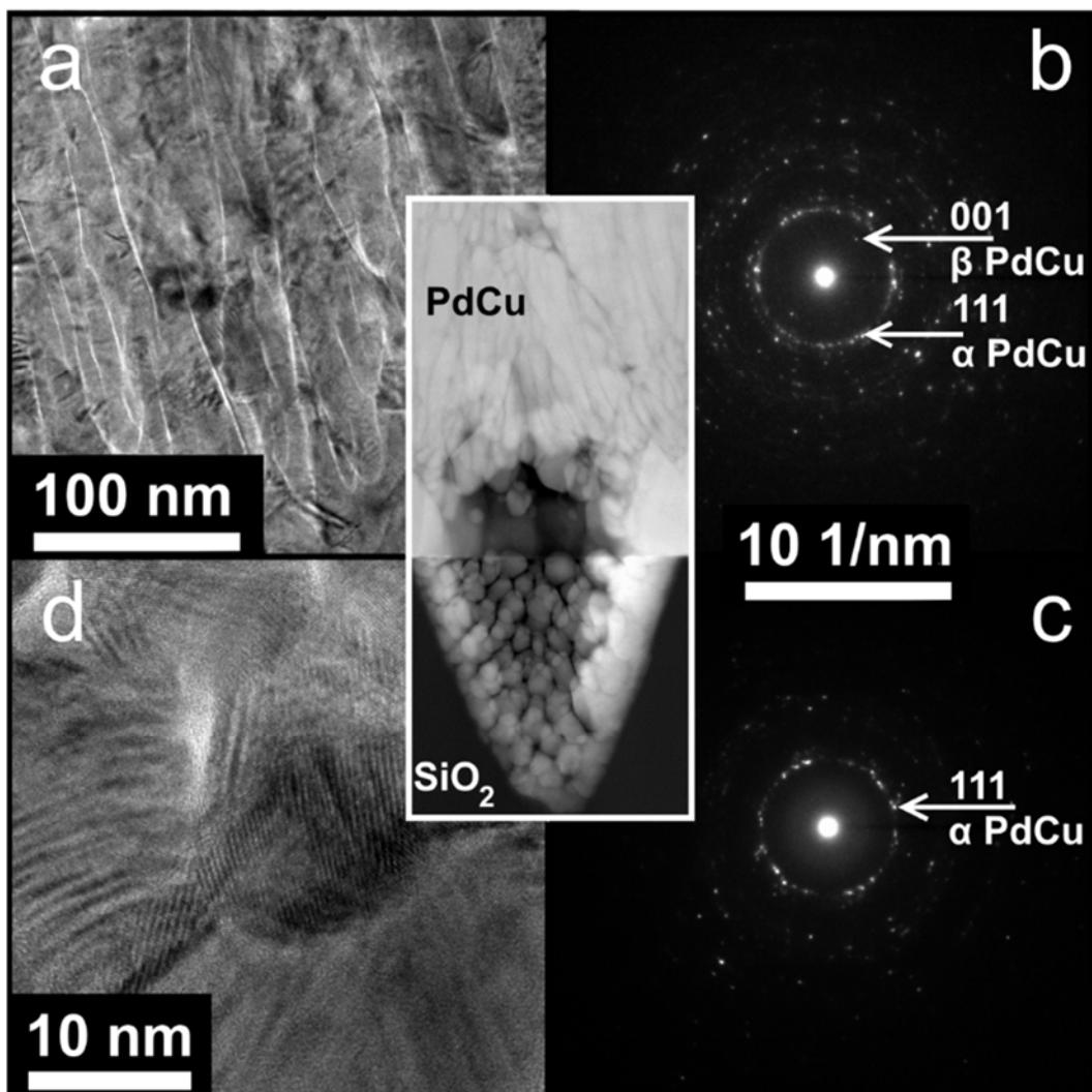
Fig. 3 Fragments of the SAED (b, c) and TEM image of the structure (a, d) cross FIB section of PdCu crystallites in the region remote from the interphase boundary with  $\text{SiO}_2$  (c, d) and inside the pore (a, b). Sample type II.
