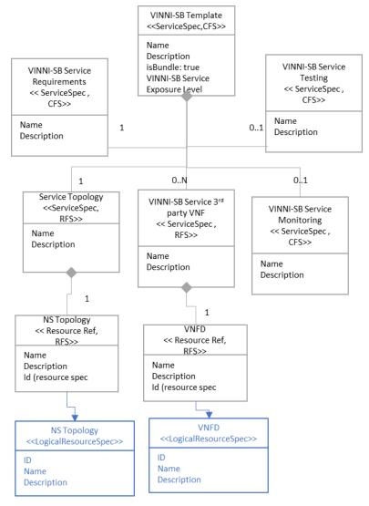
Figure 3 – The 5G-VINNI-SB Template Model diagram
