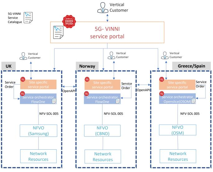
Figure 1 – 5G-VINNI architecture to enable network as a service delivery model
