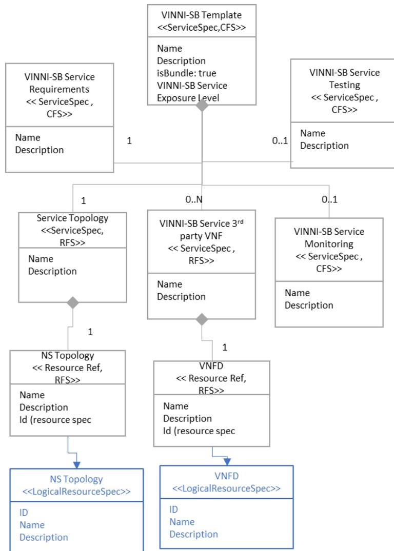
Figure 3 – The 5G-VINNI-SB Template Model diagram
