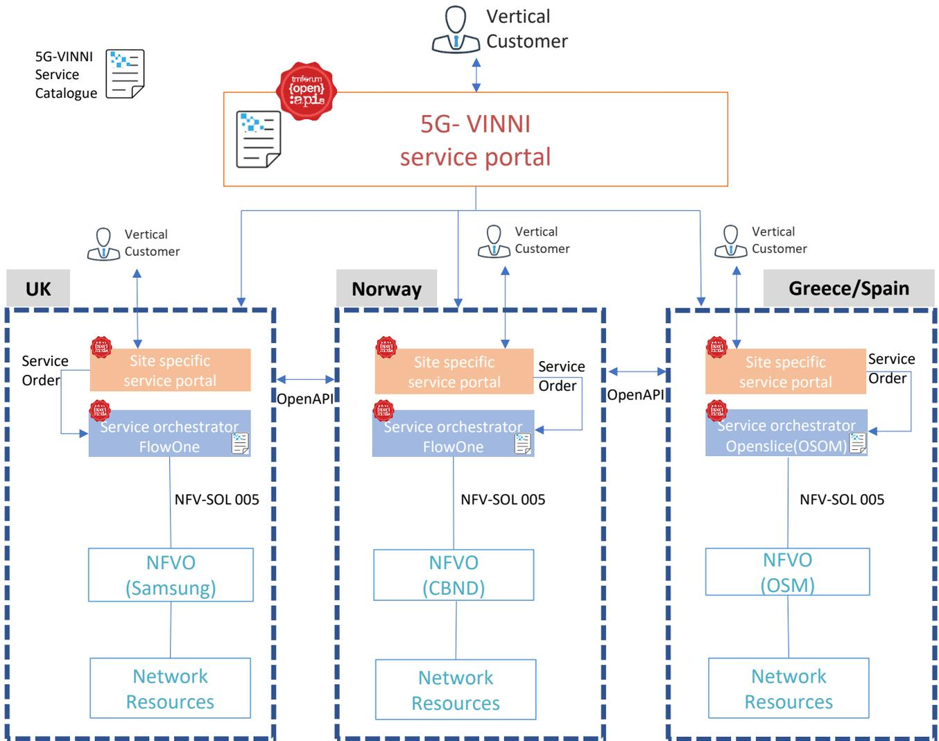
**Figure 1 – 5G-VINNI architecture to enable network as a service delivery model**
