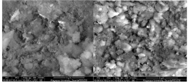
Figure 7, showed the FESEM micrograph of the sample synthesized HAP Nanoparticle (using Carica papaya leaf extract as solvent). The morphology of synthesized HAP Nanoparticle shows the agglomerated and resolved particle is represented in figure. the morphology of the particle seems to be spongy and agglomerated structure.
