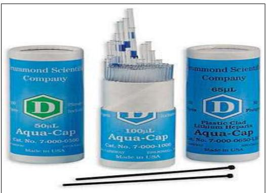
**Fig 1:-** Glass graduated 100µL capillary rods.
