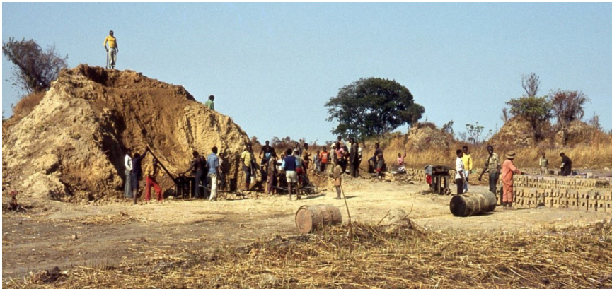
Fig. 21. — The termite mound located on the left furnishes the bricks. © L. Lemaire (†).
