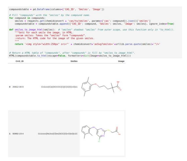
Figure 5: Chemical structures extracted through ChemIdConverter in a Jupyter notebook
