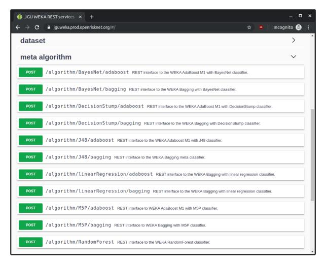
Selecting an algorithm entry opens the details for the particular algorithm. Clicking the "Try it out" button allows the user to upload a dataset or provide a URI and run the algorithm for the given data. The interface provides default values for the different parameters required for the selected algorithm. Here, we are using the default values.
