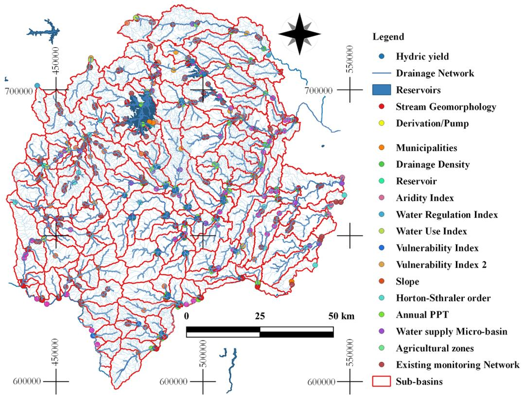
**Figure 3** Points of interest for hydrometric monitoring
