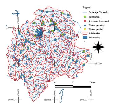
**Figure 9** Proposed hydrological monitoring network, blue triangles for water quantity stations, yellow circles for quality stations, red squares for sediment, and green star points are integrated stations (all components)
