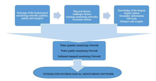
Figure 1 General methodology proposed for the redesign of the monitoring network (quantity, quality, and sediments)
