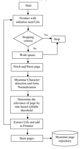
Figure 3. The design of proposed crawler
