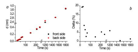
Fig. 4. (a) Dependence of the pore diameter and (b) deviation from average diameters value on the etching time.
