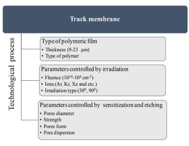
Fig. 1. Factors affecting on the characteristics of TMs.
